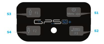
Figure 1.2: GPS SD+ keypad
